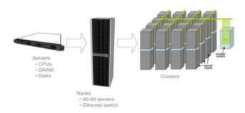
The coordination of these nodes is managed by a software layer that allows the end-user to see the cluster as a single machine. This distributed architecture allows for parallel computing and hence provides a **high level of accessibility**. The failure of one node does not affect the entire system. The system also offers greater **horizontal scalability**. An additional node can be added to the system at any time to increase its power.
